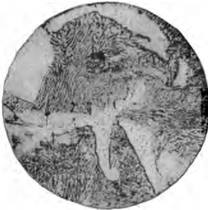
FIG. 180.—White Cast Iron. Magnified 500 Diameters. (Wust.)
